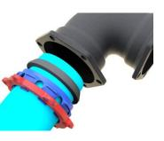
1) Clean the socket & pipe plain end. Lubricate gasket O.D. and/or socket and gasket I.D. and/or pipe plain end with soapy water or approved pipe lubricant meeting ANSI/AWWA C111/A21.11. Place the TruGrip restraint onto the pipe with the lip extension toward the pipe plain end followed by the gasket with the narrow edge of the gasket toward the pipe plain end.
