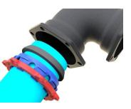
1) Clean the socket & pipe plain end. Lubricate gasket O.D. and/or socket and gasket I.D. and/or pipe plain end with soapy water or approved pipe lubricant meeting ANSI/AWWA C111/A21.11. Place the TruGrip restraint onto the pipe with the lip extension toward the pipe plain end followed by the gasket with the narrow edge of the gasket toward the pipe plain end.
