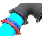
2) Insert the gasket along with the pipe into the fitting socket and seat or press in the gasket firmly and evenly into the gasket cavity, keeping the joint straight and aligned.
