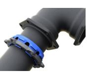
2) Insert the gasket along with the pipe into the fitting socket and seat or press in the gasket firmly and evenly into the gasket cavity, keeping the joint straight and aligned.
