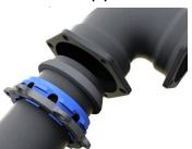
1) Clean the socket & pipe plain end. Lubricate gasket O.D. and/or socket and gasket I.D. and/or pipe plain end with soapy water or approved pipe lubricant meeting ANSI/AWWA C111/A21.11. Place the TruGrip restraint onto the pipe with the lip extension toward the pipe plain end followed by the gasket with the narrow edge of the gasket toward the pipe plain end.
