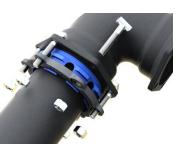
3) Push the TruGrip restraint toward the fitting socket and center it around the pipe with the lip extension evenly and firmly against the seated gasket. Insert the T-head bolts with the T-head on the fitting side. For proper assembly, snuggly hand tighten all nuts before using a driver. Make any joint deflection after hand tightening the nuts and before applying further torque. Maximum deflection is 3 degrees for (4"-12") pipe diameters
