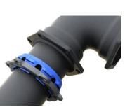
2) Insert the gasket along with the pipe into the fitting socket and fully seat or press in the gasket firmly and evenly into the gasket socket, keeping the joint straight and aligned.
