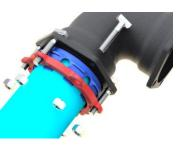
3) Push the TruGrip restraint toward the fitting socket and center it around the pipe with the lip extension evenly and firmly against the seated gasket. Insert the T-head bolts with the T-head on the fitting side. For proper assembly, snuggly hand tighten all nuts before using a driver. Make any joint deflection after hand tightening the nuts and before applying further torque. Maximum deflection is 3 degrees for (4"-12") pipe diameters
