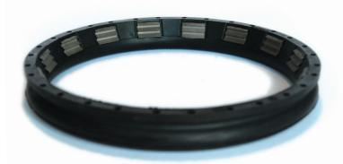
GASKETS are produced and tested in accordance with ANSI/AWWA C111/A21.11 and have a 350 psi pressure rating. The gaskets have been successfully tested at a minimum of 700 psi to nationally recognized listing agency requirements, as witnessed by independent testing agencies (certificates available upon request).
